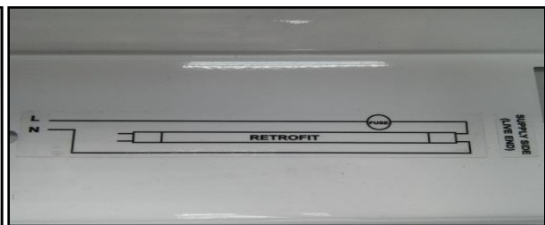
Connector Block with Inline Fuse (High melting point of 125°C which make it a safe fuse to use)
